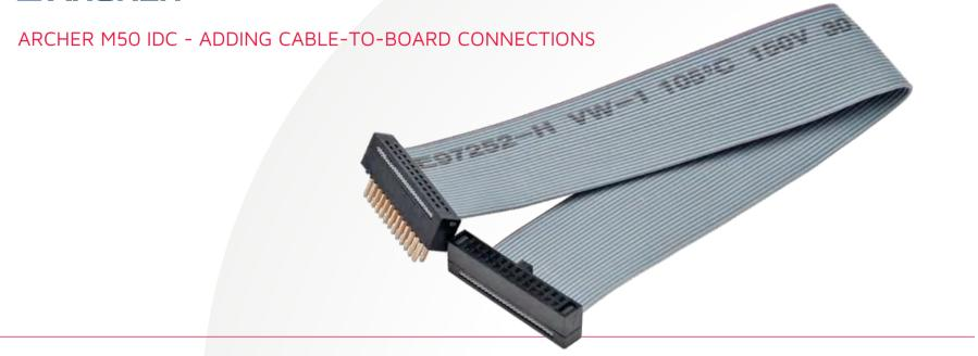
The Archer M50 range has additional cable-to-board options, by utilising Insulation Displacement Connectors (IDC) to provide a <u>cable connection</u> to 0.635mm pitch flat ribbon cables. IDC contacts make connection to the wire conductor cores by cutting through the insulation as part of the process of wire assembly to the connector. Therefore, no wire stripping is required, making the connectors a fast, single-operation connector.
