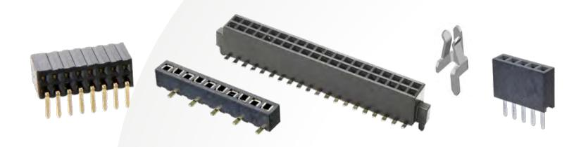
The M50 range of the Archer connectors are all based on a 1.27mm pitch grid (1.27mm pitch both along the connector, and between the two rows), and male pins are 0.4mm square. Single and Double row are available.
