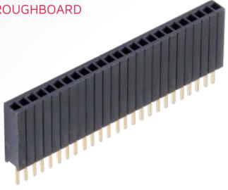
The Archer M52 range include both single and double row options, based on a 1.27mm pitch along the connector. Pitch between rows on the double row is 2.54mm, and male pins are 0.46mm square.
