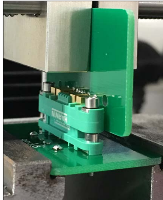
Figures 1 & 2: Examples of the test setups for board-to-board durability testing using an automatic force gauge (HWN 4162).
