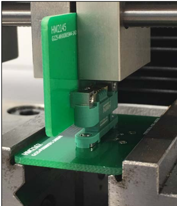
Figures 1 & 2: Examples of the test setups for board-to-board durability testing using an automatic force gauge (HWN 4162).
