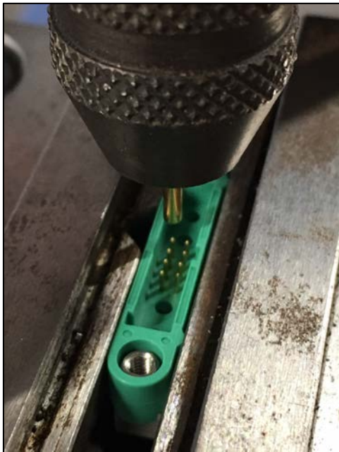
Figure 1: Pin used for contact removal testing from PCT assembly on automatic force gauge (HWN 4162).
