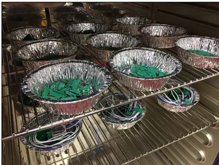
Figure 3: Individual connectors and mated assemblies arranged within the testing oven (HWN 3592) for 96hrs, 250hrs and 1000hrs temperature life.
