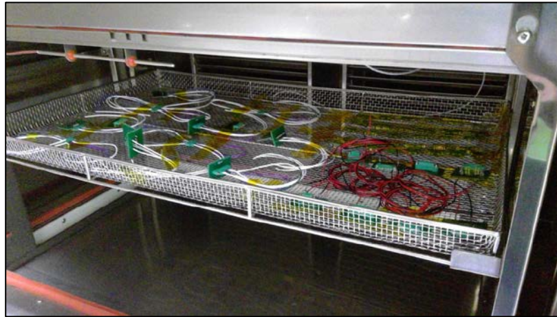
Figure 5: Samples in thermal shock chamber
