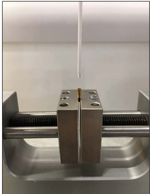
Figure 4: 18AWG test sample with the wire being pulled from the crimp area.
