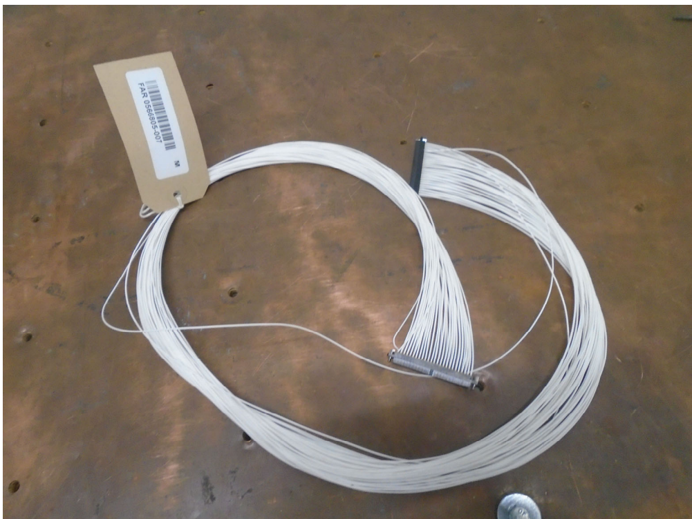
Figure 1.3.5 Equipment Under Test - 50-way cable unshielded
