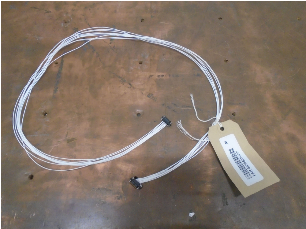
Figure 1.3.1 Equipment Under Test - 10-way cable unshielded
