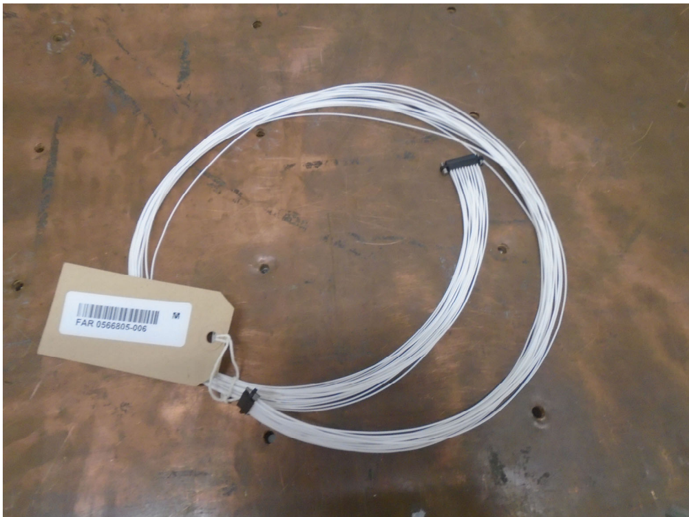
Figure 1.3.3 Equipment Under Test - 20-way cable unshielded
