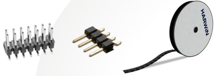
The Surface Mount Pin Headers come in both Vertical and Horizontal configurations. Each can be supplied in tape and reel packaging format to facilitate automated assembly processes to the PCB. Vertical SMT connectors in tape and reel will be fitted with disposable pick-and-place caps.
