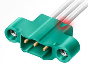
All male and female connector bodies carry a triangular-shaped inset in the housing, to indicate the position of the Number 1 contact. Counting is then continued along the row. For Double row connectors, the numbering restarts on the second row from the contact beside position 1, and continues along the row as before.
