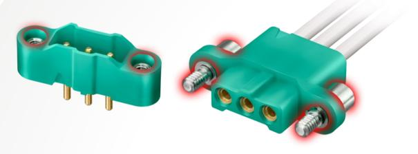
Female crimp connectors are fitted with floating Hex Socket jackscrews, suitable for 2mm Hex (Allen) keys. These will engage with jackscrews assembled in both Male PC Tail and Male Crimp connectors.
