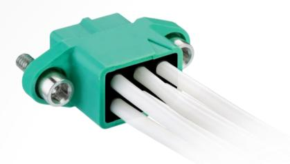
The crimp housings feature a potting wall to keep potting fluids retained during application. The use of potting improves the retention of the crimp contacts in the housing by adding strain relief. The ready-made cable assemblies come with backpotting in place.
