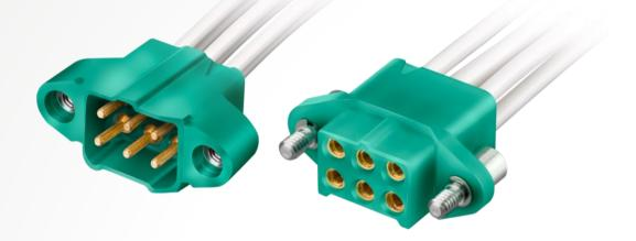
Both Male and Female cable connectors are designed to suit 18AWG to 22AWG equipment wires, with a maximum external diameter of Ø1.8mm for 18-20AWG, and Ø1.4mm max for 22AWG.
