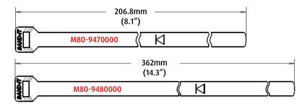
For Datamate connectors, the BAND-It tie has always been sold separately. If your backshell and braiding exceed 22.4mm at the widest point, we recommend you switch to using the longer M80-9480000 tie.
