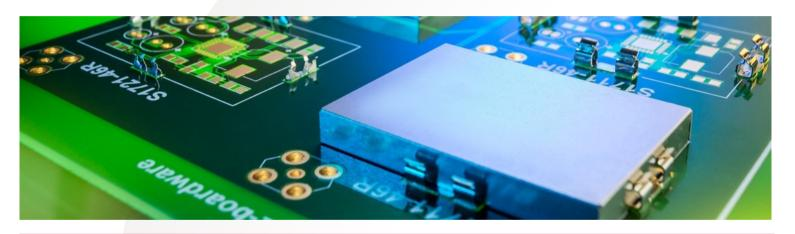
A soldered can that covers components requiring rework must first be desoldered. The remedial work underneath is carried out, then the can must be soldered back in place. Each solder operation adds the risk of damage, and greatly increases the rework cost due to time and operator skill.
