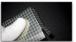
The Shield Can Kit S01-806005KIT allows you to make prototypes and limited quantities of cans, quickly and easily. The blanks are simple to cut and easy to form, requiring no special tooling. Pre-scored on a 5mm grid, cans of 5mm, 10mm or higher are possible. Maximum can size per sheet is 70mm x 50mm, 5mm high.
