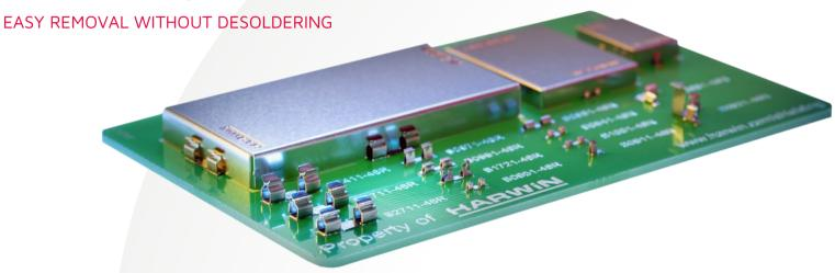
Harwin's SMT Clip and Can system works by soldering the Clips to the PCB during the SMT phase. The Cans are then pushed into the clips in a very quick secondary operation.
