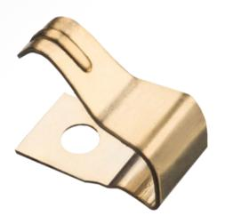
A development of the 'C' style contact, this design uses a more obvious cantilever style. The SMT pick and place area is exaggerated to compensate for the miniature size of the contact. This range is provided in 0.5mm incremental step heights, from 2mm up to 5mm. The footprint is the same across the complete set of contacts.
