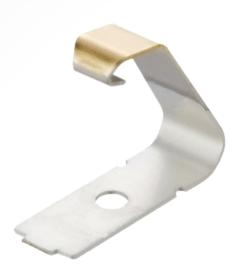
The 'C' style contact is the simplest of designs, providing a flexible connection between PCBs, components and chassis grounds. Manufactured from copper alloy, they provide excellent spring properties over extended periods of time.
